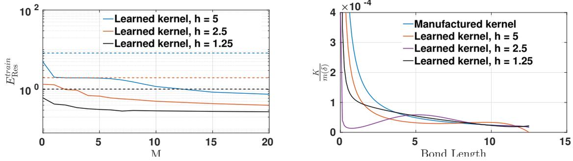
Figure 2: Consistency tests for Algorithm 1 with fixed  $\alpha = 1$  and positive influence function. Left: The training loss versus basis order  $M$  when using different grid size; the dashed lines indicate the values of the loss functions when the manufactured kernel is used, colors reflect the values of  $h$  used for discretization. Right: The comparison of learned influence functions and the manufactured influence function  $K_{\text{man}} = \frac{1}{r}$ .
