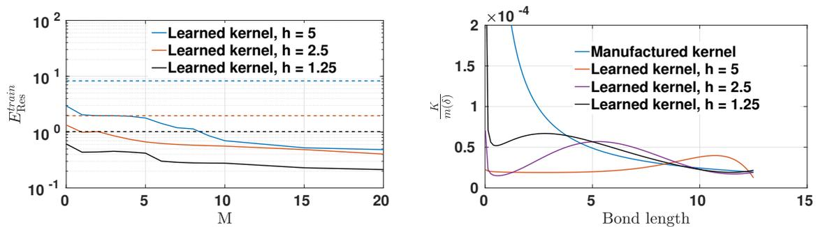
Figure 3: Consistency tests for Algorithm 1 and positive influence function, while learning  $\alpha$ . Left: The training loss versus basis order  $M$  when using different grid size; the dashed lines indicate the values of the loss functions when the manufactured kernel is used, colors reflect the values of  $h$  used for discretization. Right: The comparison of learned influence functions and the manufactured influence function  $K_{\text{man}} = \frac{1}{r}$ .
