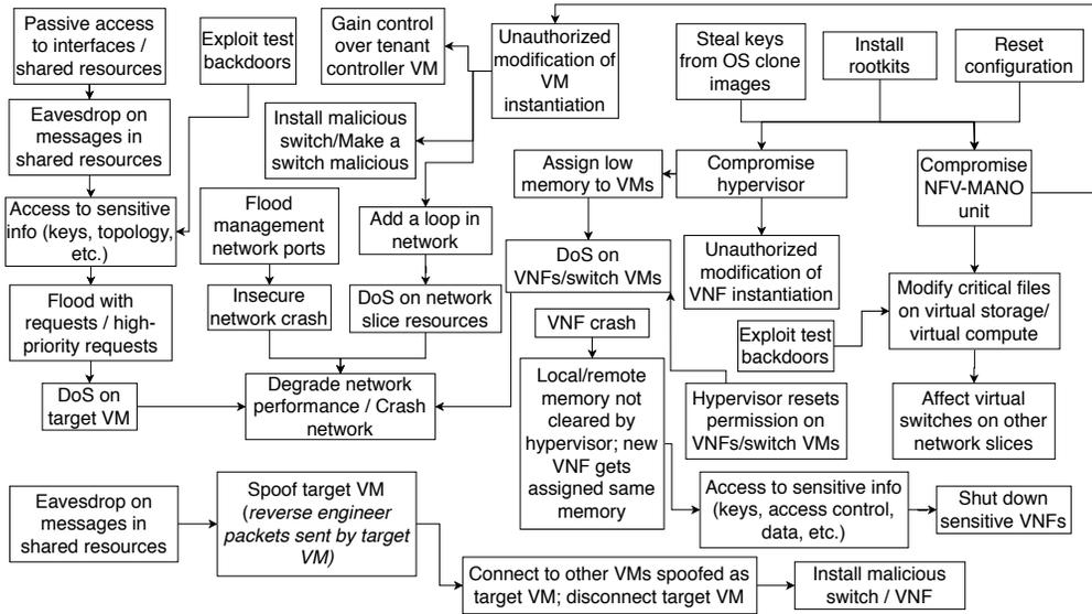
Fig. 7: Aggregated attack graph of NFV vulnerabilities
