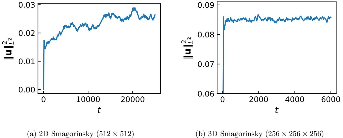
FIGURE 1. Evolution of the energy of the reference solution over the transient period.
