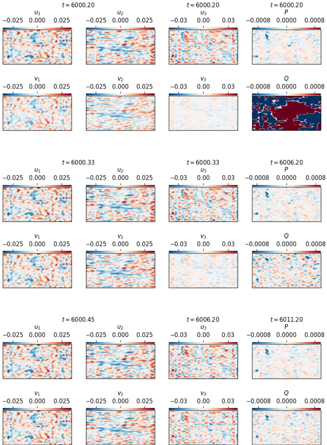
FIGURE 8. Abridged data assimilation for the 3D Smagorinsky model with  $(\mu_1, \mu_2, \mu_3) = (10, 10, 0)$  and  $h = h(128)$ . These are the slices on the mid-plane  $(0, 2\pi) \times (0, 2\pi) \times \{z = \pi\}$ . Note the time progression is different for different components of velocity and pressure.
