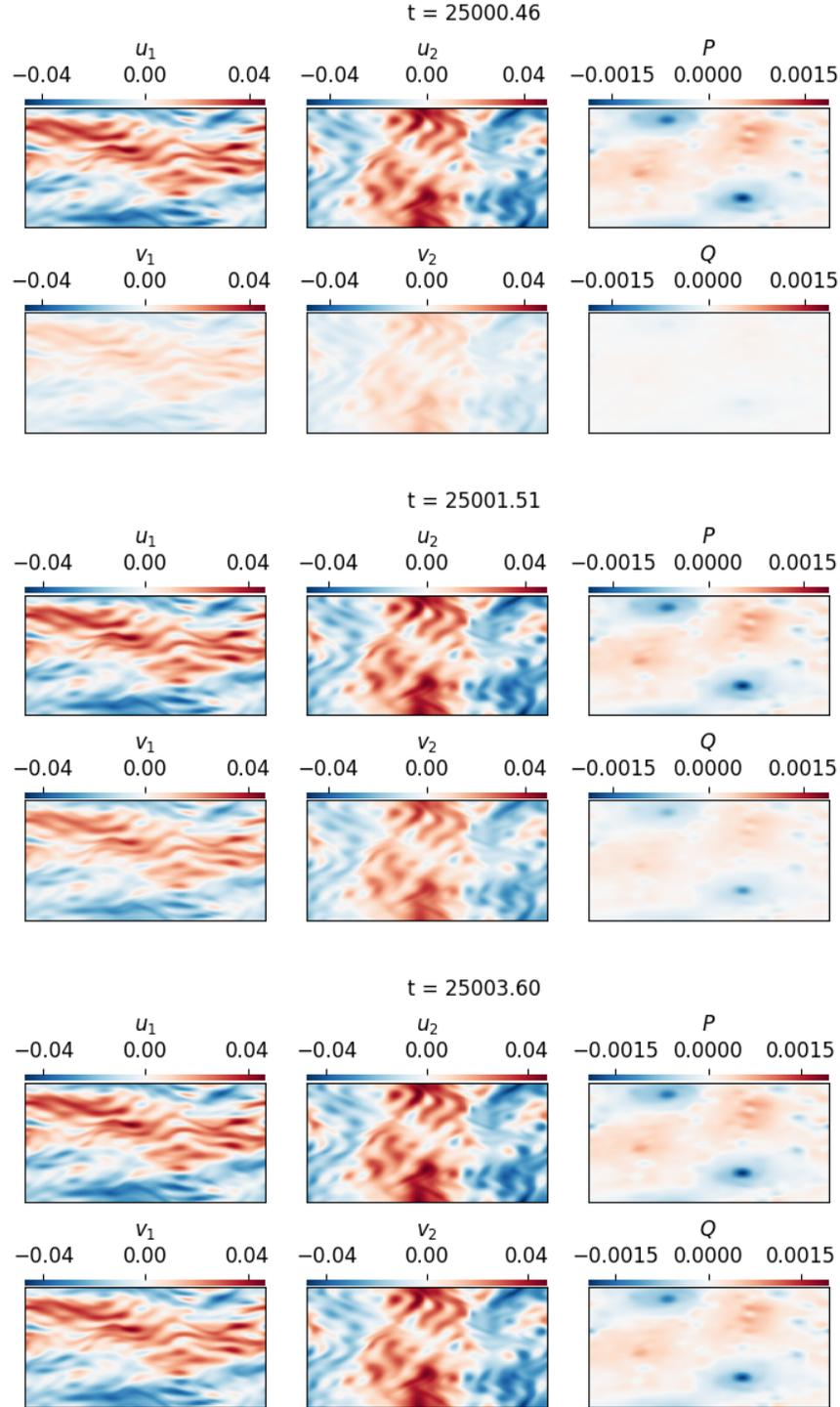
FIGURE 4. Synchronization of the 2D Smagorinsky model using nodal interpolation,  $\mu = 1$  and  $h \approx 0.0491$ ; the reference solution  $(\mathbf{u}, P)$  is denoted as  $(u_1, u_2, P)$  and the nudging solution  $(\mathbf{v}, Q)$  is  $(v_1, v_2, Q)$ .
