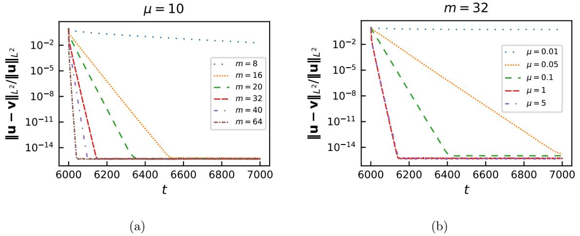
FIGURE 3. Convergence of data assimilation for the 3D Smagorinsky at different values of the nudging parameter  $\mu$  and  $h = h(m)$ ; the left fixes  $\mu = 10$  and the right fixes  $m = 32$ .
