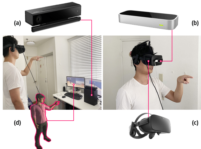
Fig. 3: Device arrangement. The human player wears an (c) Oculus headset with (b) Leap Motion. (a) Kinect is placed 1.5m from the human player and 1.5m above the ground. The screen displays (d) A humanoid model that are mirroring the body and hand movements.
