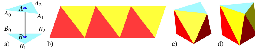
Fig. 1 The antiprismatic skeleton for n = 3 (a), its belt given by the Kresling pattern (b), the resulting octahedral structure (c) and its configuration after the snap (d).
