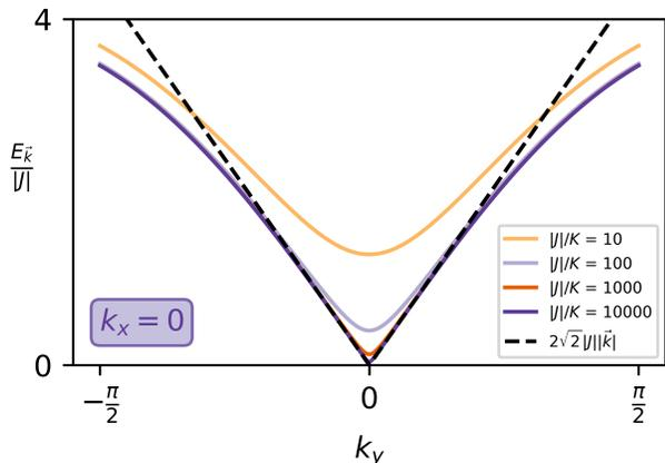
FIG. 6. Ratio of energy and  $|J|$  for different values of  $|J|/K$  and  $J = -1$  showing the lowering of the energy gap for smaller  $K$  and the approach to a linear dispersion. Dashed black line gives the linear dispersion with  $\varepsilon_{\vec{k}}/|J| = 2\sqrt{2}|\vec{k}|$ .
