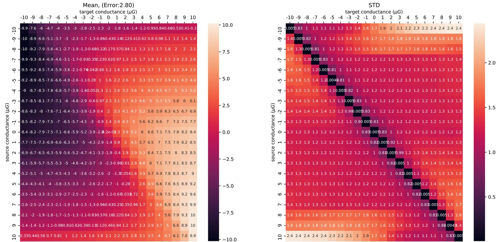
Figure 10: Multi-memristor configuration with 8 PCM (four depression and four potentiation) per synapse
