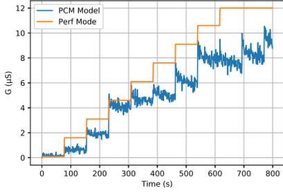
(a) Comparison of the full PCM model and its `perf`-mode equivalent after 8 consecutive SET pulses.
