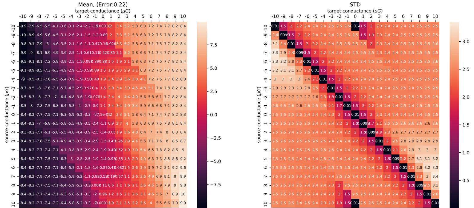
Figure 12: Update-ready criterion tested with  $N = 1$  memristor per synapse.
