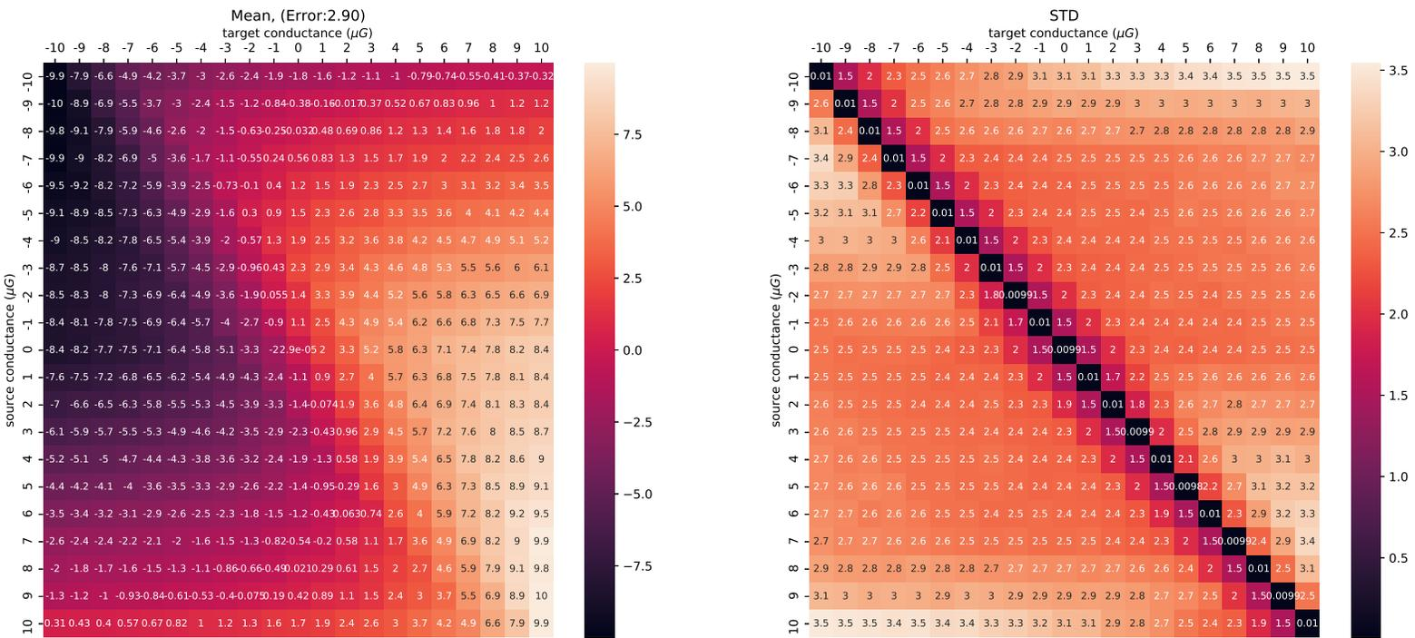
Figure 9: Multi-memristor configuration with 1 PCM (one depression and one potentiation) per synapse
