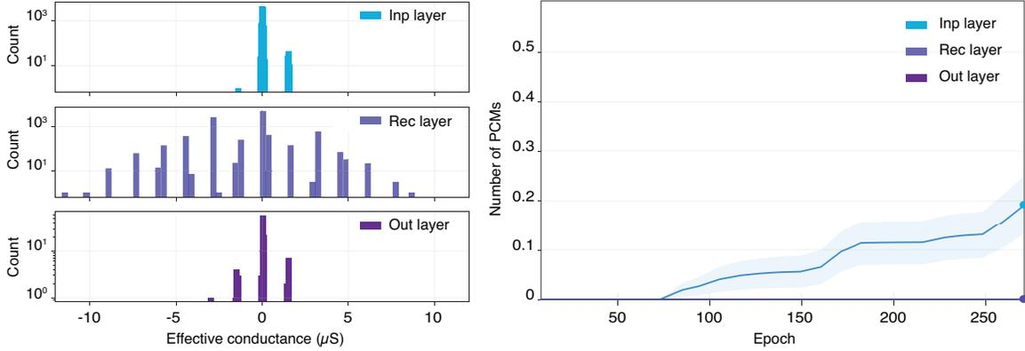
Figure 5: (left) The effective conductance distributions ( $G^+ - G^-$ ) of the synapses in the input, recurrent and output layer, at the end of the training with the mixed-precision method. (right) Averaged over 50 training runs, the mean number of PCM devices requiring a refresh is shown for each layer. The refresh operation was not needed for recurrent and output layers.
