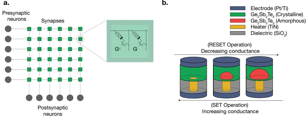
Figure 1: **a.** PCM devices can be arranged in a crossbar architecture to emulate both a non-volatile synaptic memory and a parallel and asynchronous synaptic propagation using in-memory computation. **b.** Mushroom-type geometry of a single PCM device. The conductance of the device can be reconfigured by changing the volume ratio of amorphous and crystalline regions.
