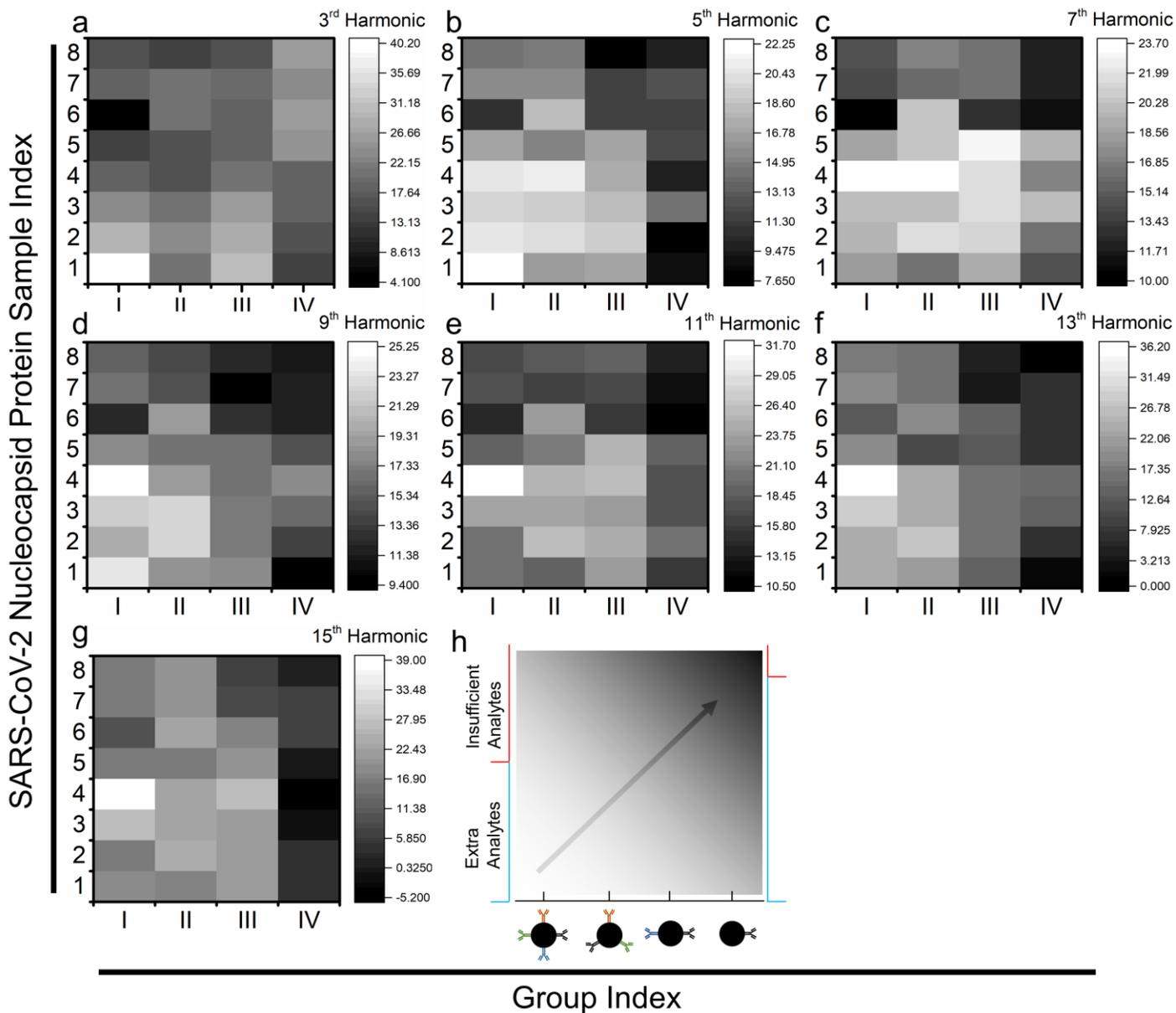
**Figure S5.** Grayscale heatmaps of higher harmonic signal drop  $\Delta$  (in %) compared to bare MNPs for SARS-CoV-2 nucleocapsid proteins.
