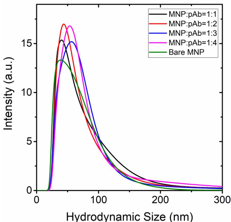
**Figure S3.** The hydrodynamic size distributions of bare MNPs, MNPs each functionalized with one, two, three, and four pAbs.
