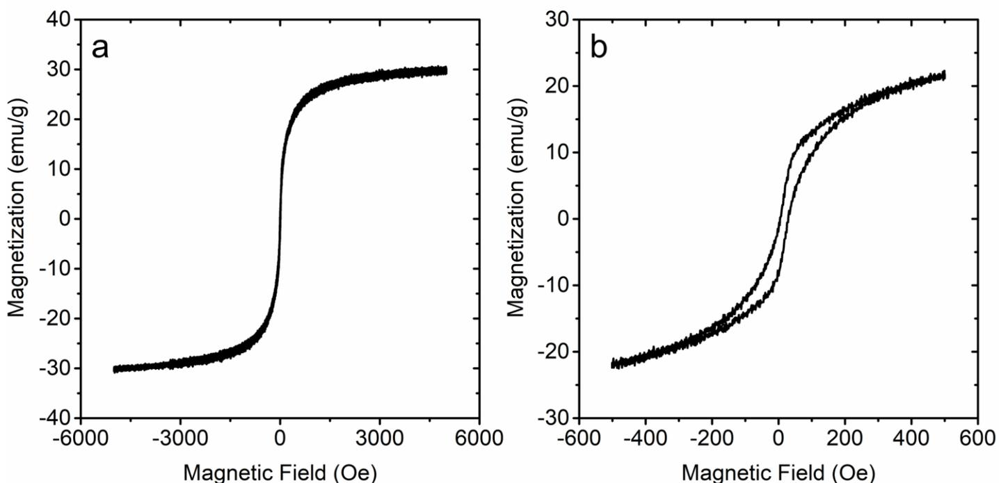
**Figure S1.** Static magnetic hysteresis loops of air-dried IPG30 MNPs measured by a PPMS. The field range is (a) -5000 – 5000 Oe and (b) -500 – 500 Oe, respectively.
