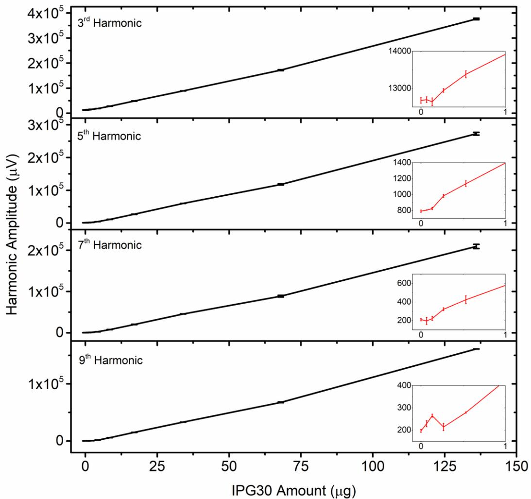
**Figure S2.** The higher harmonic amplitudes collected from vials 1-13 with varying amount of IPG30 MNPs. Error bars represent standard errors.
