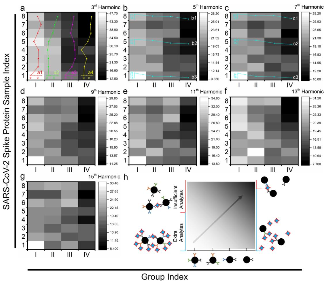
**Figure S4.** Grayscale heatmaps of higher harmonic signal drop  $\Delta$  (in %) compared to bare MNPs for SARS-CoV-2 spike proteins. (a) – (g) are the 3<sup>rd</sup>, 5<sup>th</sup>, 7<sup>th</sup>, 9<sup>th</sup>, 11<sup>th</sup>, 13<sup>th</sup>, and 15<sup>th</sup> harmonic signal drop from 32 samples in Group I – IV compared to bare MNPs, respectively. (a1 - a4) are the harmonic signal drop,  $\Delta$ , plotted as a function
