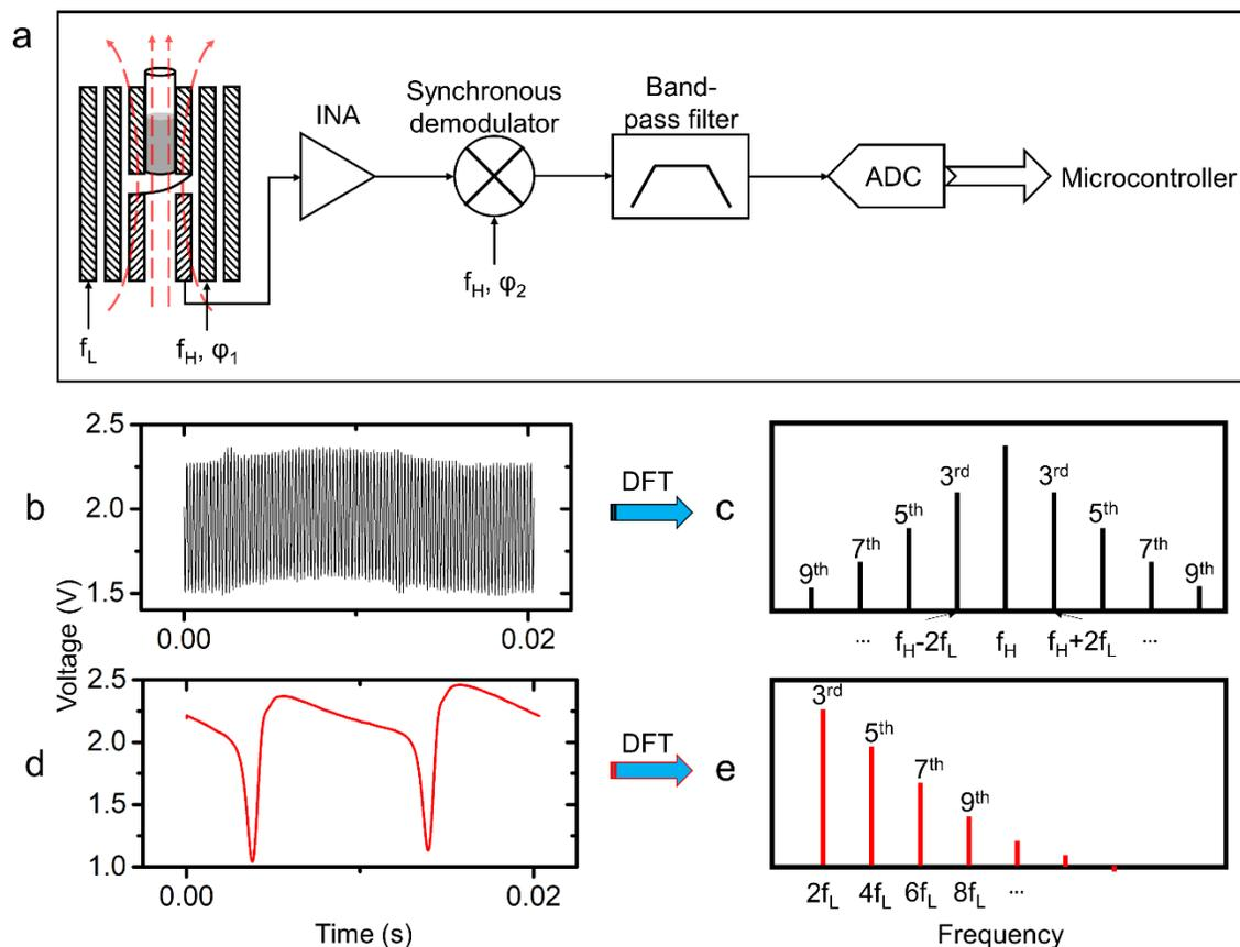
**Figure 1.** (a) Schematic diagram of the MPS system with a one-stage lock-in implementation. (b) is the time-domain voltage signal collected from pick-up coils after INA amplification stage and (d) shows the voltage signal post lock-in implementation. (c) and (e) are the MPS spectra from (b) and (d) after discrete Fourier transform (DFT), respectively.
