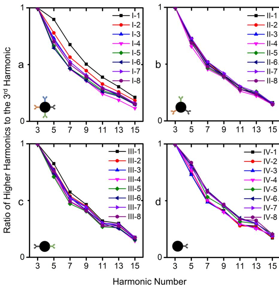
Figure S6. Ratios of higher harmonics to the 3<sup>rd</sup> harmonics recorded from Groups (a) I, (b) II, (c) III, and (d) IV. For SARS-CoV-2 nucleocapsid protein detection.
