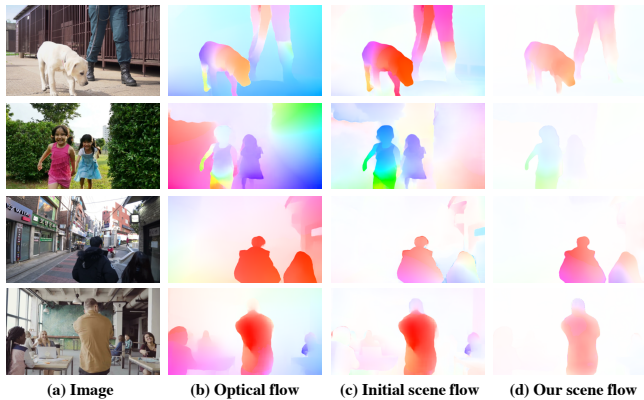
Fig. 7. Scene flow results. Colors correspond to the direction of the projected flow, while saturation corresponds to magnitude (white is zero flow). Optical flow (b) contains both background and foreground motion. Projected scene flow derived from the initial depth estimate (c) and optical flow (b) has small, but still noticeable motion in stationary areas. Our projected scene flow (d) is concentrated in the truly moving regions of the scene.
