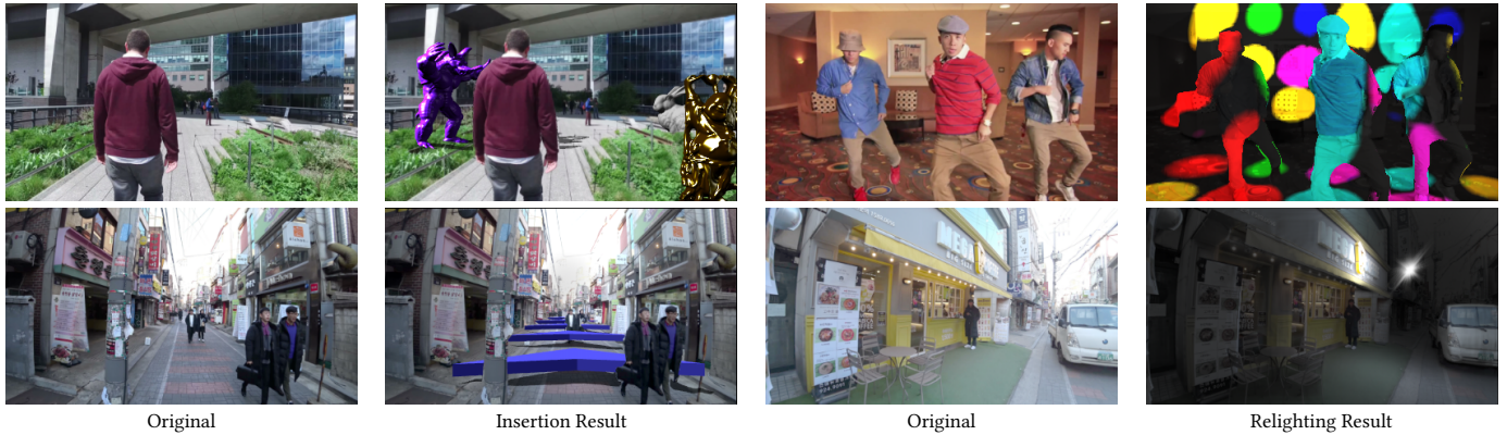
Fig. 9. Object and light insertion. Because of their temporal coherence, the depth buffers produced by our method may be used to insert objects (top) or position-dependent lighting effects (bottom) without distracting flickering. Please see supplemental material for a video comparison with single-frame depth prediction.
