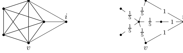
Figure 3: A mesh-star transformation of K_5 to S_6 with d_i = 3
