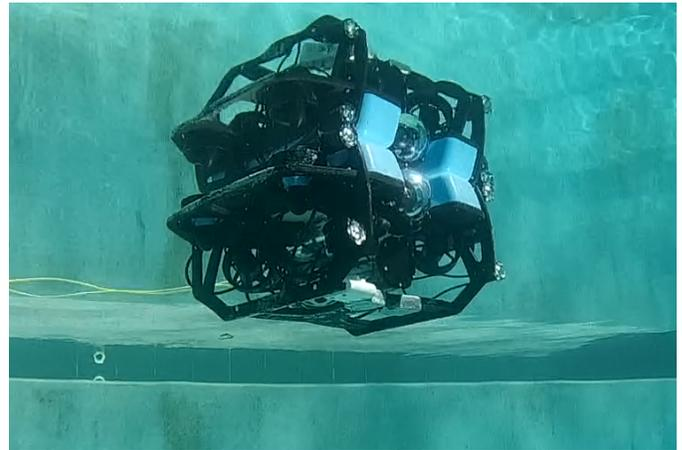
Fig. 1. A modified BlueROV2 used for experiments
