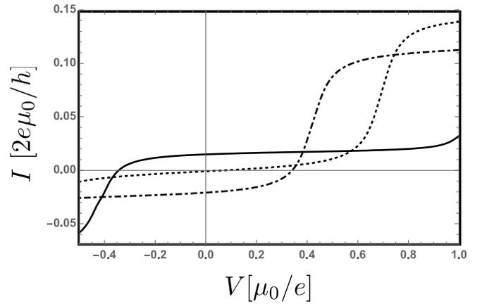
FIG. 2.  $I - V$  characteristics in the non-linear regime for  $T_h = 2$  K;  $T_c = 0.05$  K,  $\varphi = 2\pi\Phi_{AB}/\Phi_0 = \pi$ ,  $\mu_0 = 10^{-22}$  J,  $\varepsilon = 0.1$ , and  $\delta\tau = 0.3$ . The curves correspond to  $V_g = 0.63$  mV (solid),  $V_g = 1.1$  mV (dashed), and  $V_g = 1.5$  mV (dash-dotted). Thermovoltages for different  $V_g$  correspond to the crossing points with the  $x$ -axis, *i.e.* for  $I = 0$ .
