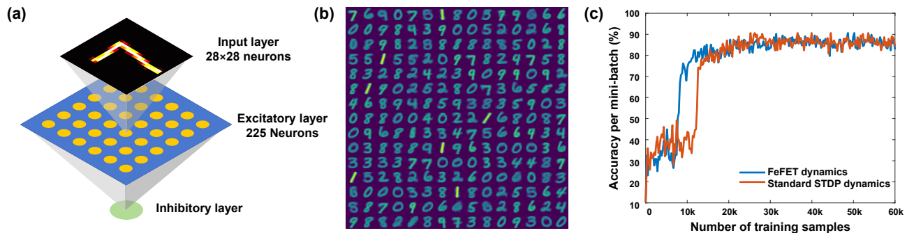
FIG. 5. (a) Our SNN architecture consists of an excitatory neuron layer with lateral inhibitory connections for unsupervised learning. The synaptic weights joining the input and excitatory layer are implemented using FeFET devices and undergo STDP learning. (b) FeFET synaptic array conductance states after training on the MNIST dataset for the 225-neuron network. (c) Accuracy per mini-batch during training with respect to the number of training samples. We observed a sharp rise in accuracy as the network activity decreased and weights became learnt. Further updates mostly fine-tuned the weights. It can be seen that this convergence in learning occurs with 33.3% fewer training samples while using the FeFET dynamics compared to the standard STDP learning rule.
