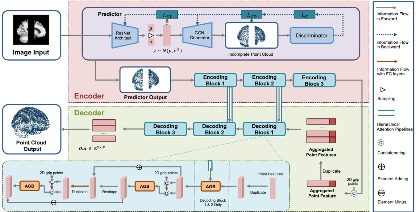
Fig. 1. The architecture of the proposed model. The pink area is the encoder network, composed of a predictor and three encoding blocks based on PointNet++. In addition to outputting the extracted features to the next block, the first two encoding blocks also feed them back to the corresponding decoding block through the attention pipeline. The green area represents the decoder network. The detailed structure of the decoding block is also given in the blue room.
