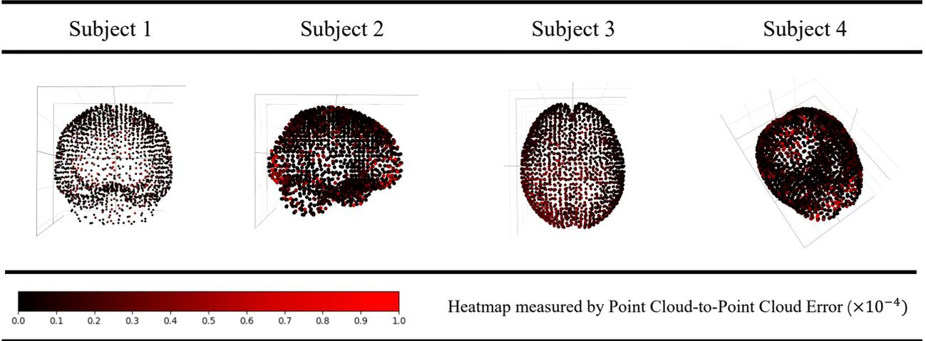
Fig. 6. The point-to-point reconstruction accuracy results in multiple of angles which is represented by the heat map colored by PC-to-PC error.
