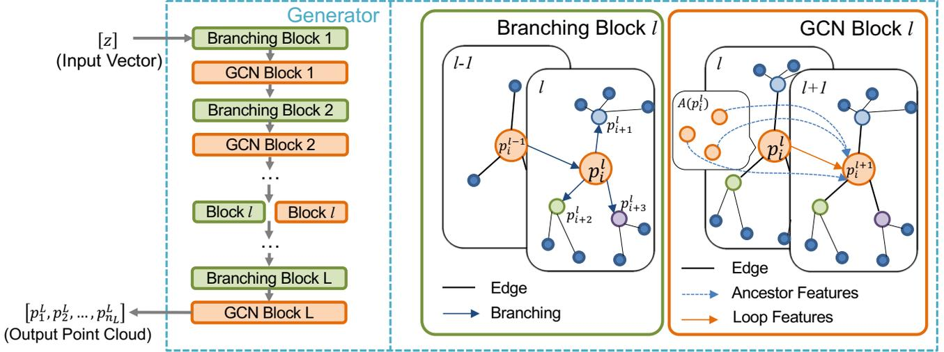
Fig. 2. The detailed structure of the generator in the predictor. An improved branching graph convolution network consisting of multiple GCN block and branching block groups is constructed.
