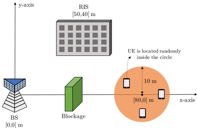
Fig. 5. The location of the BS, the RIS, and the UE throughout simulation.
