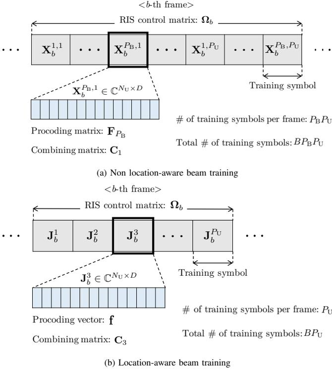
Fig. 3. A frame structure for non location-aware beam training and location-aware beam training in RIS-aided MIMO communication.
