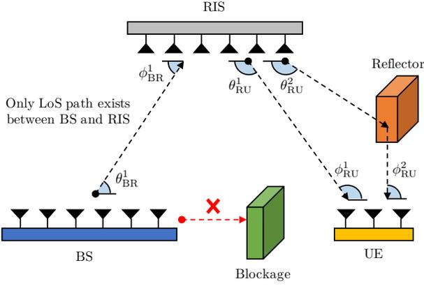
Fig. 1. A scheme of RIS-aided mmWave MIMO system and propagation paths. The signal path between BS and UE is blocked.
