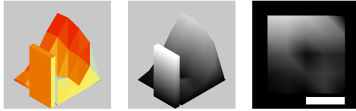
Fig. 4. From left to right: i) optimized geometry with solar radiation colors – SE Isometric, ii) optimized geometry with depth map – SE Isometric, iii) top view projection of (ii) – final format of data.
