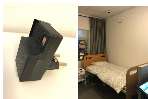
Fig. 1. Left: Griddy with the Panasonic Grid-EYE infrared array sensor on the front. Right: Bed used in data collection with Griddy in the ceiling.
