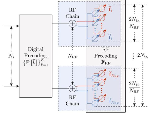
**Fig. 1.** Hybrid analog/digital precoding architecture in a mmWave band MIMO-OFDM system with cross-polarization.
