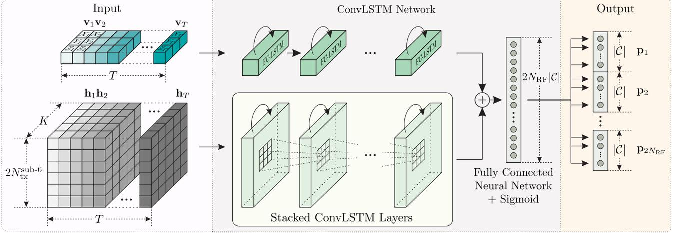
**Fig. 2.** The proposed neural network architecture for beam prediction/tracking. The network takes the spatiotemporal sub-6GHz channel measurements with  $T$  samples in sequence and predicts the mmWave beam indices in  $T + 1$  time step.
