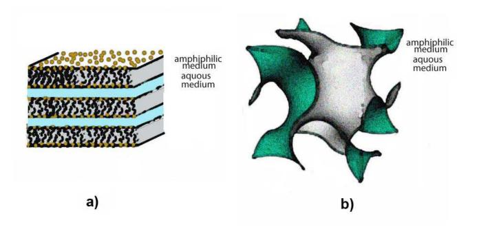
FIG. 1: a) Schematic representation of the lamellar phase of a lyotropic liquid crystal, amphiphilic flat layers are separated by water layers; b) schematic representation of a cubic phase (gyroid surface), two interwoven but not connected labyrinths of water channels are separated by a single film of amphiphilic molecules with an intricate topology. In the lamellar phase layers have a null curvature when the gyroid surface has a negative Gaussian curvature.
