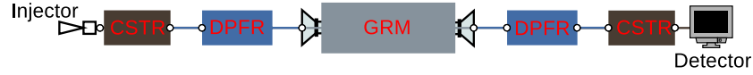
Figure 1: Schematic of mathematical models used to describe transport behaviour between injector and detector of a chromatography equipment. Lines do not represent tubings, instead just connection. External dispersion effects between injector and column are described with DPFR; external volume effects are described with CSTR. Mass transfer in the column is described with GRM. Models between column and detector are mirrored in this study.
