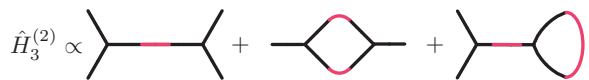
FIG. 6. Diagrammatic representation of \hat{H}_3^{(2)} . The first diagram gives a correction to the Kerr term ( \hat{a}^\dagger \hat{a}^2 ) as it has four uncontracted legs. The last two diagrams have two uncontracted legs and yield corrections to the frequency. The placement and number of Wick contractions (red lines) agrees with the contractions that occur during normal ordering, cf. Eq. (C4). We have omitted a diagram that is proportional to the identity, i.e., all legs are contracted, as it does not contribute to the dynamics.
