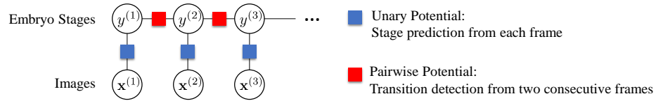
Fig. 2. Linear-Chain CRF Model. For each image, we compute the unary potential using a image model. For pairwise ones, we use predictions from a transition detector.
