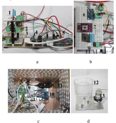
Fig. 3. Electrical part farm 1 - board with sensors, 2,3 - analog boards for signals processing, 4 - power board, 5 - battery, 6 - CO2 sensor, 7 - illumination sensor, 8 - temperature sensor, 9 - RaspberryPI3, 10 - battery board, 11 - LED, 12 - vessel for water, 13 - pump
