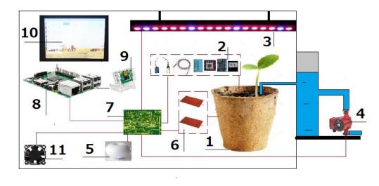
Fig.2. The farm operation scheme: 1 - crop, 2 - sensors, 3 - LED, 4 - pump, 5 - humidifier, 6 - air and soil heaters, 7 - analog digital converter, 8 - RaspberryPI, 9 - camera, 10 - operator panel, 11- fan.
