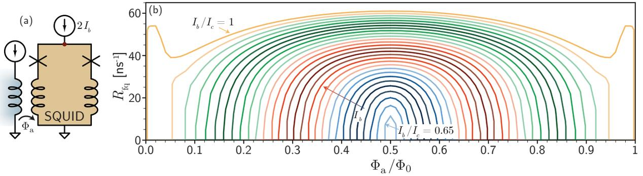
Figure 1: (a) SQUID circuit with DC current bias ( $I_b$  through each JJ) and flux input ( $\Phi_a$ ) through a transformer. (b) SQUID response function.  $R_{fq}$  is the rate of flux-quantum production due to the voltage developed at the node indicated by a red dot in part (a) as a function of the applied flux to the SQUID loop in units of the magnetic flux quantum  $\Phi_0 = h/2e$ . Different curves correspond to different bias conditions.
