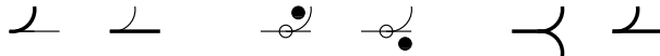
Figure 7 The switches used in the railway circuit of the model. To left, the fixed switch, in the middle, the flip-flop switch, to right the memory switch. In the flip-flop switch, the bullet indicates which track has to be taken.
