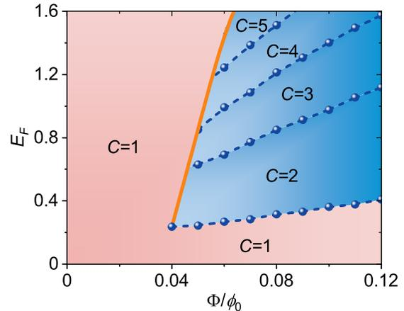
FIG. 4. (color online) Phase diagram of a disordered ferromagnetic insulator  $\text{MnBi}_2\text{Te}_4$  in the  $E_F - \Phi/\phi_0$  plane. The blue balls mark the extended states of Landau bands and the solid line indicates the phase boundary. The phase diagram is identified from the renormalized localization length  $\Lambda_M$ .
