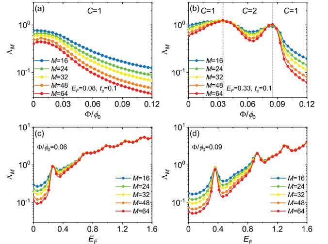
FIG. 3. (color online) (a) and (b) Renormalized localization length  $\Lambda_M = \lambda(M)/M$  against the magnetic field  $\Phi/\phi_0$  with different Fermi energies. (c) and (d) display  $\Lambda_M$  as a function of Fermi energy under different magnetic field strengths. The calculation is performed with the periodic boundary condition in the x direction.
