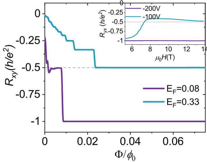
FIG. S1. (a) Calculated Hall resistance  $R_{yx}$  as a function of magnetic field  $\Phi/\phi_0$  under different Fermi energies. (b) Calculated longitudinal resistance  $R_{xx}$  and  $R_{yx}$  as a function of Fermi energy. The insets show the experimental measured  $R_{xx}$  and  $R_{yx}$  adopted from Ref. [1], where  $\mu_0 H$  and  $V_g$  correspond to the magnetic field and Fermi energy, respectively. The numerical simulation is performed with sample size of  $400 \times 400$  sites.
