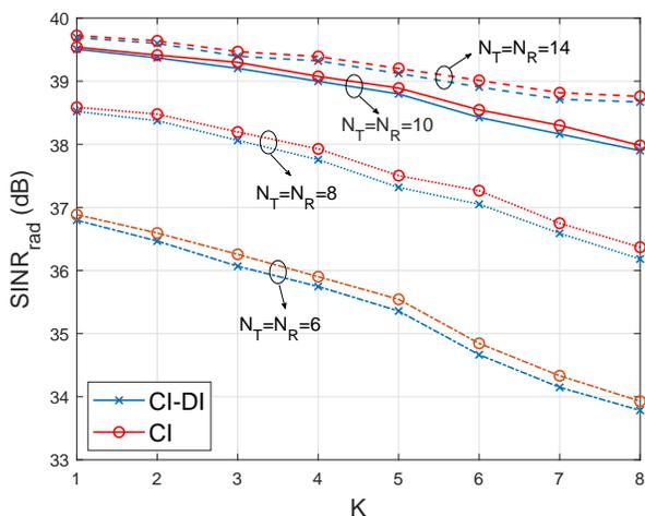
Fig. 8. The received SINR of radar versus the number of CUs with different number of DFRC BS antennas.
