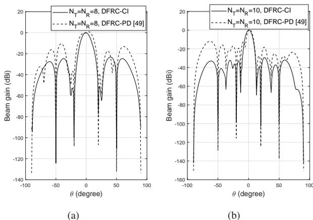
Fig. 4. Optimized beam patterns with different number of DFRC BS antennas, here, the beamformer design approach proposed in [49] is set as benchmarks,  $K = 5$ .
