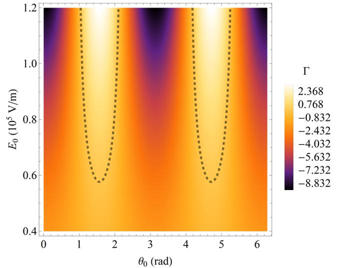
FIG. 7. Contour plot of the ratio  $\Gamma$  for the cesium atom varying  $\theta_0$  and  $E_0$ . The dashed black line indicates combinations of  $\theta_0$  and  $E_0$  for which  $\Gamma = 0$ . Here, we chose  $R = 60$  nm and  $a = 700$  nm.
