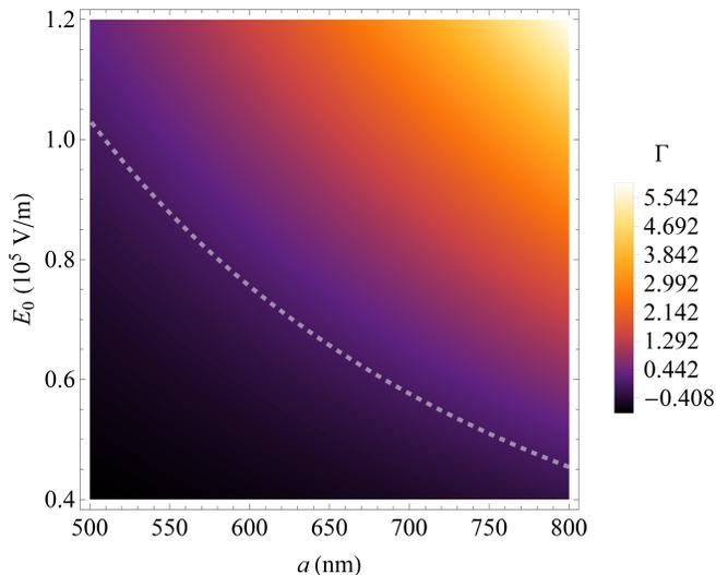
FIG. 8. Contour plot of the ratio  $\Gamma$  for the cesium atom varying  $a$  and  $E_0$ . The dashed white line indicates combinations of  $a$  and  $E_0$  for which  $\Gamma = 0$ . Here, we chose  $R = 60$  nm and  $\theta_0 = \pi/2$ .
