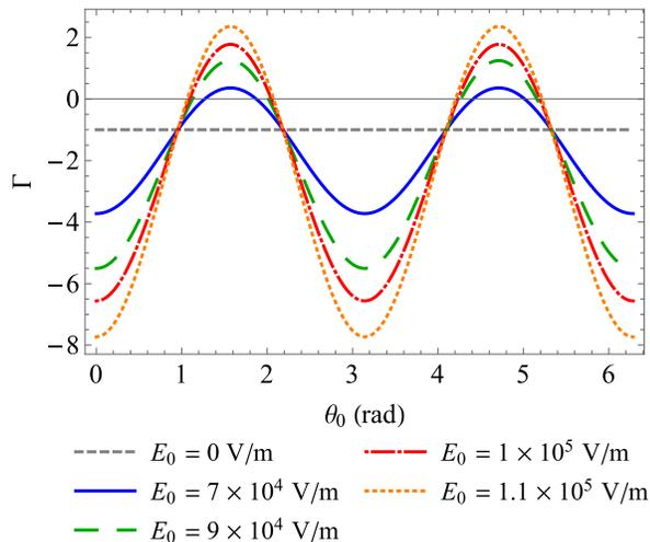
FIG. 2. Ratio  $\Gamma$  as a function of the angle  $\theta_0$  between the applied electric field and the  $Oz$ -axis. Different colors refer to different field intensities. We set  $R = 60$  nm and  $a = 700$  nm.
