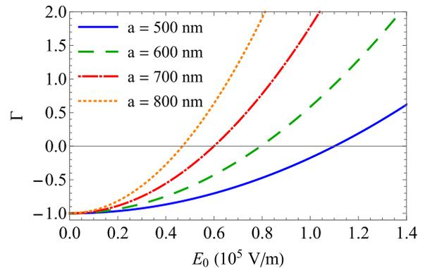
FIG. 3. Ratio  $\Gamma$  as a function of the field intensity  $E_0$ . Different colors denote different distances  $a$  from the atom to the sphere's surface. We set  $R = 60$  nm and  $\theta_0 = \pi/2$ .
