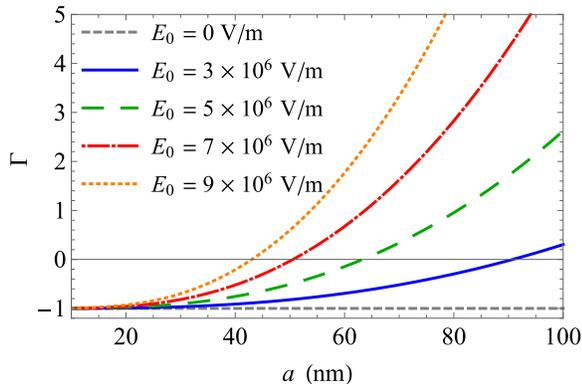
FIG. 5. Ratio  $\Gamma$  as a function of the distance  $a$  from the atom to the sphere's surface for different field intensities in the short-distance regime. We set  $R = 60$  nm and  $\theta_0 = \pi/2$ .
