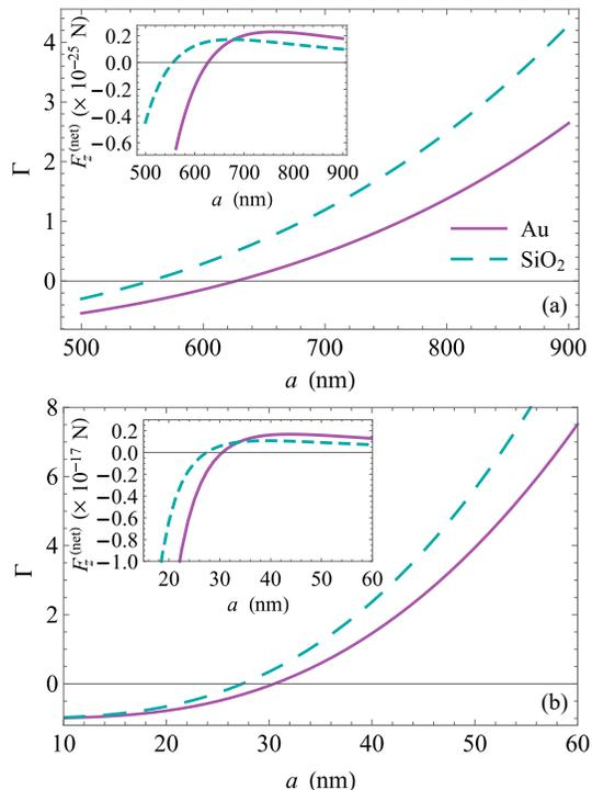
FIG. 9. Ratio  $\Gamma$  as a function of the distance  $a$  between a cesium atom and the sphere's surface for **(a)**  $E_0 = 7 \times 10^4$  V/m, using Eq. (1), and **(b)**  $E_0 = 9 \times 10^6$  V/m, using Eq. (6). In all panels, different colors refer to spheres made of different materials, and we set  $R = 60$  nm and  $\theta_0 = \pi/2$ . The insets show the resultant force on the atom as a function of  $a$ .
