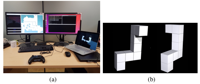
Fig. 1. 1a: The experimental apparatus: the Operator Control Unit (OCU) composed of a laptop, a joypad, a mouse and a screen showing the GUI; and a laptop presenting the secondary task. 1b: A typical example of the secondary task [24].
