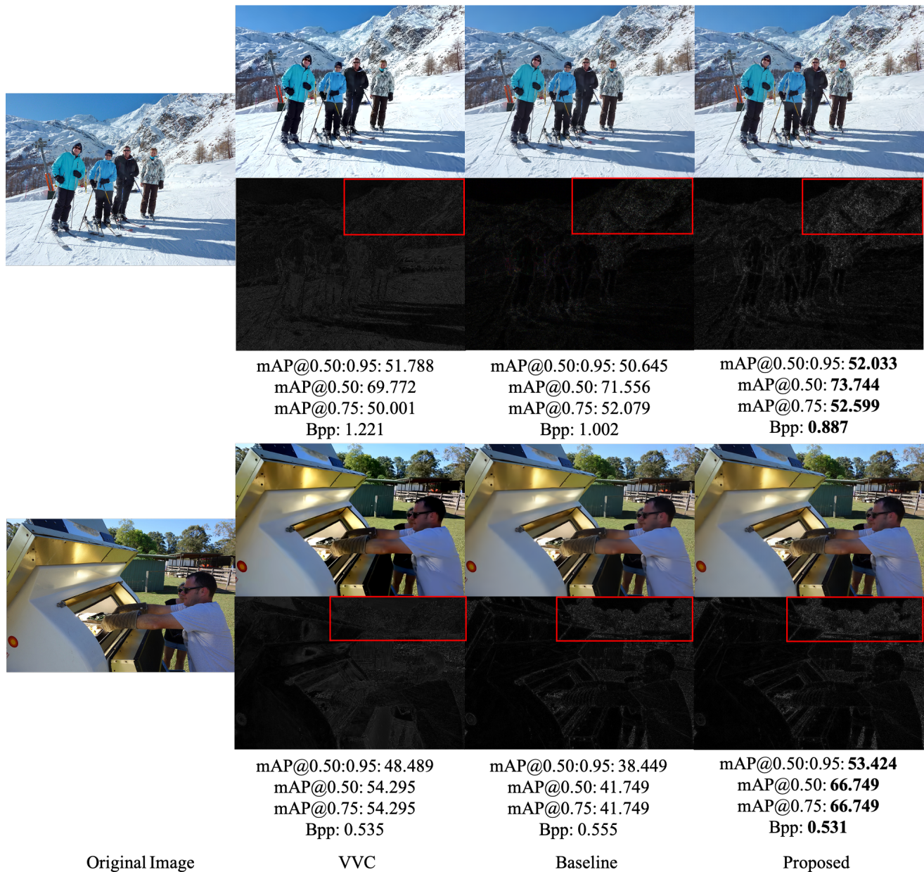
Fig. 9. Visualization of the reconstructed images of the proposed framework, compared with the VVC and baseline model. For every compression codec, the MAD between the reconstructed and the original images are visualized with min-max normalization, accompanying with the bitrate and the analysis accuracy. The red rectangles indicate the regions that are compressed aggressively, as they are not particularly important in the analysis task.
