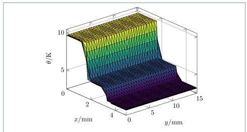
Figure 8: Temperature distribution in the Rutherford cable at  $z=z_{\rm q}=0.33\,{\rm m}$  at time  $t=10\,{\rm ms}.$
