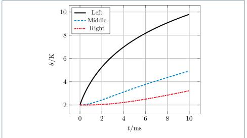
Figure 6: Evolution of the temperature in the three cables over time. Evaluated at  $z=z_{\rm q}$  and in the center of the cross-section of each cable.
