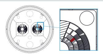
Figure 1: Cross-section of cos-theta magnet for Future Circular Collider (FCC) and High-Energy Large Hadron Collider (HE-LHC). A stack of three Rutherford cables is highlighted in red [13].
