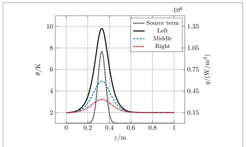
Figure 7: Temperature distribution in z-direction in the three cables at time  $t=10\,\mathrm{ms}$  and the source term in dependency of z. The temperature of the cables is evaluated in the center of their cross-section.
