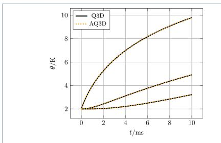
Figure 13: Evolution of the temperature in the three cables over time calculated with the Q3D and AQ3D method. Evaluated at  $z=z_{\rm q}$  and in the center of the cross-section of each cable.
