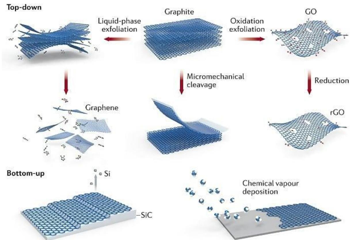
Fig 3. Various synthesis methods of graphene<sup>21</sup>.
