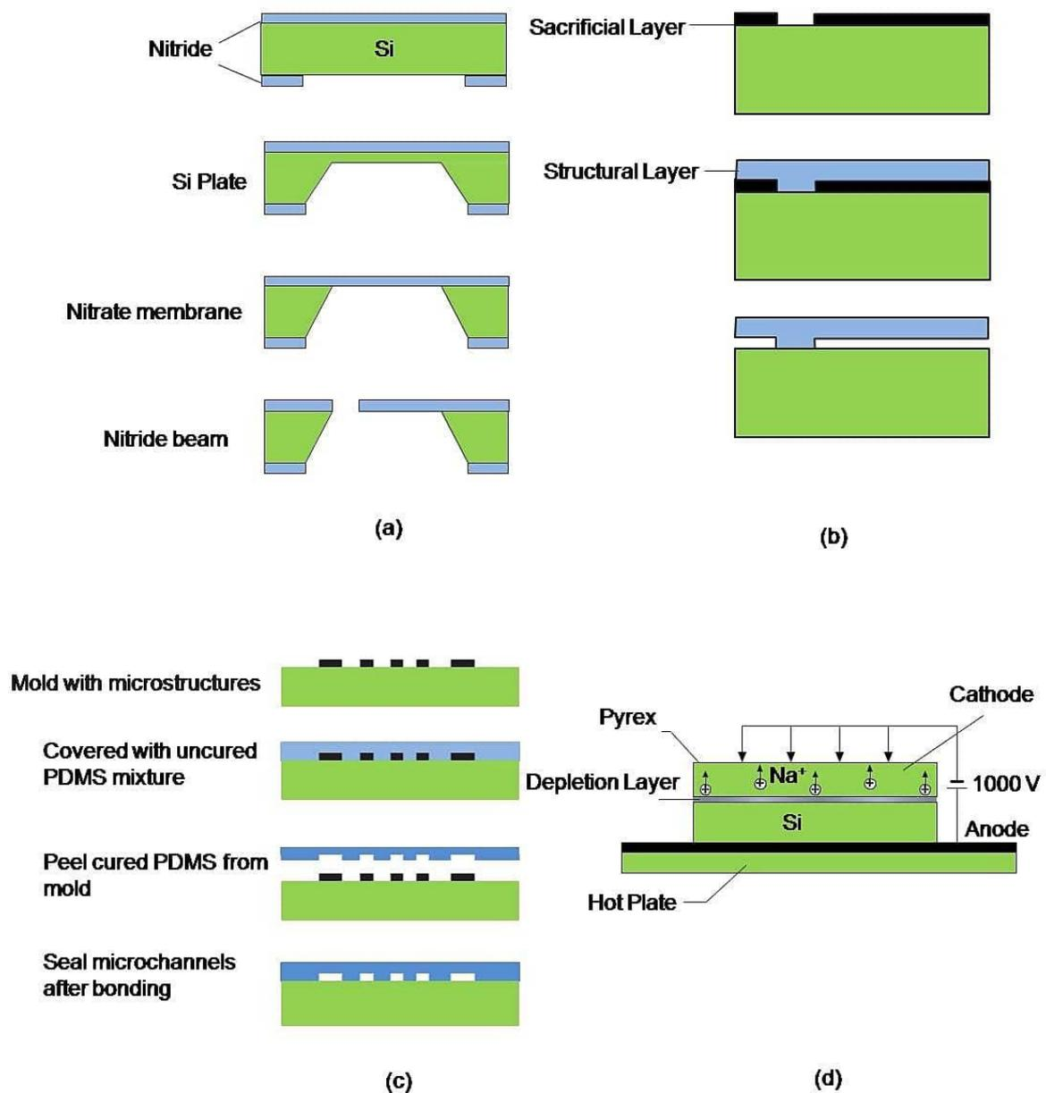
Fig 1. Different routes LOC fabrication: a) Bulk Micromachining, b) Surface Micromachining, c) SoftLithography, d) Bonding<sup>8</sup>.
