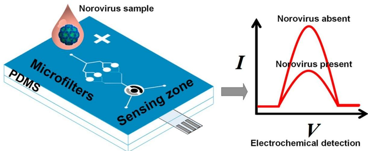
Fig 7. Microfluidic carbon electrode with Grp-AuNPs composite for Norovirus detection<sup>101</sup>.
