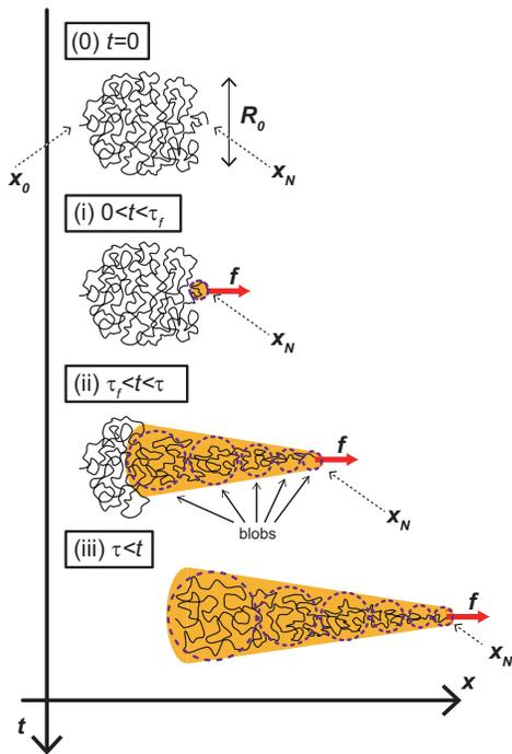
FIG. 1. (Color online) Schematic representation of polymer stretching. (0) initial equilibrium coil. (i) early blob formation for  $0 < t < \tau_f$ . (ii) stretching transient for  $\tau_f < t < \tau$ . (iii) nonequilibrium steady state for  $t > \tau$ . Dashed circles represent blobs (local coilings), and an entire moving domain is shaded.
