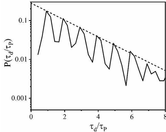
**Fig. S9.** Semi-log plot of the residence time distribution of the particle in the symmetric double-well potential in the presence of nonGaussian active noise of  $f_{act} \approx 1 \text{ pN}$  and  $\tau_c/\tau_p \approx 0.25$ . The dotted line corresponds to  $y = 0.28 \exp(-0.5x)$ . The fitting of the dotted line with the peak heights demonstrates that the height of each peak decreases exponentially with their order  $n$ .
