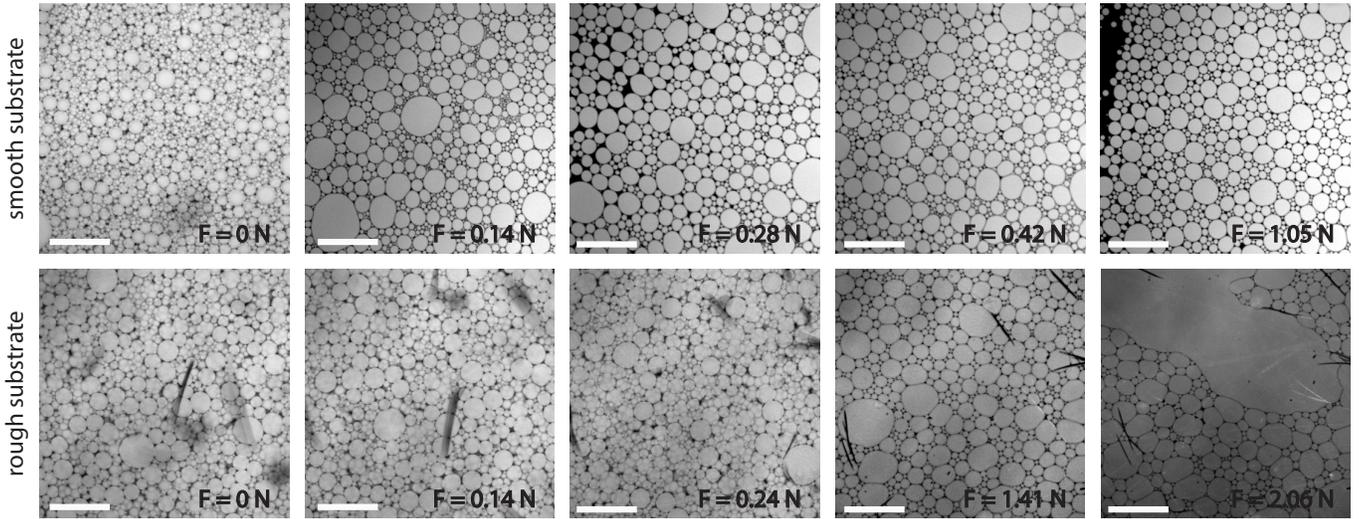
FIG. 3. Squeezing experiments on a smooth (top) and a rough (bottom) glass substrate. From left to right, the squeezing force increases from 0 to 1.05 N. Whereas the oil droplets glide over the smooth substrate, they are pinned on the rough substrate, allowing for further deformation of the droplets and finally destabilization of the emulsion. Scale bars are  $50 \mu\text{m}$ .
