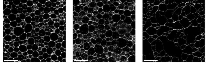
FIG. 4. BSA/PGA-stabilized emulsion destabilization by squeezing. Confocal images showing deformation of the emulsion droplets and coalescence events in the emulsion after a critical sample thickness is reached. Scale bars are  $100 \mu\text{m}$ .
