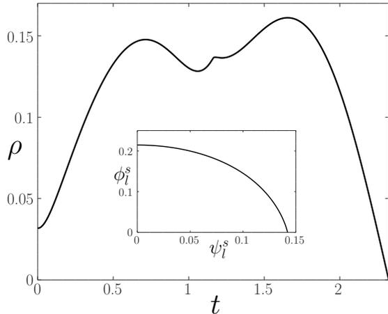
FIG. 7. Main panel: the minimum friction coefficient  $\rho(t)$ , sufficient to prevent sliding, is plotted between  $P_s$  and  $P_d$ . Inset: the parametric plot of  $\phi_l(t)$  vs  $\psi_l(t)$  for  $t \in (0, t_s)$  shows the swing foot trajectory. The finite slope at the impact indicates finite  $\rho(t_s)$ .
