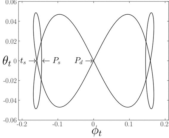
FIG. 4. The parametric plot of  $\theta_t(t)$  vs  $\phi_t(t)$  shows the torso's trajectory relative to the legs over one walking cycle for the (3,4)-mode. The Lissajous-like curve features 3 coronal and 4 sagittal oscillations. The symmetry points  $P_s$  and  $P_d$ , and the impact point (indicated here as  $t_s$ ) are denoted in the left half of the plot.
