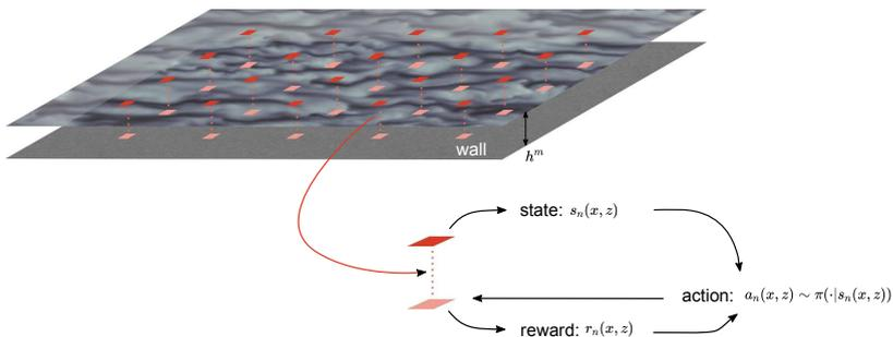
**Fig. 1 Diagram of the SciMARRL setup.** Agents are distributed evenly along the wall, with each agent obtaining state information wall-normal height  $h^m$  away from the wall, computing the reward at the wall and supplying in to the policy  $\pi$  to obtain actions  $a$  for the next time step.
