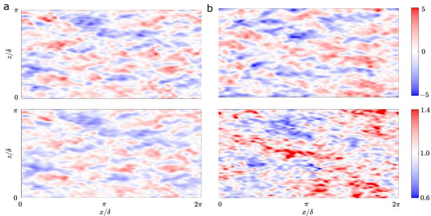
**Fig. 6 Comparison of the instantaneous off-wall streamwise velocity and wall-shear stress.** Instantaneous snapshots of  $x$ - $z$  plane of streamwise velocity fluctuation  $u'^*$  at  $h^m$  (top) and  $\tau_w^m/\tau_w$  (bottom) for (a) EQWM and (b) LLWM.
