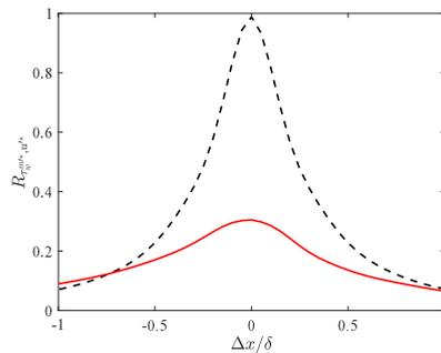
**Fig. 7 Correlation of instantaneous off-wall streamwise velocity and wall-shear stress.** Cross-correlation coefficient between the wall-shear stress  $\tau_w^{mI*}$  and streamwise velocity  $u'^*$  at sampling location  $h^m = 0.1\delta$  for LLWM (red solid line) and EQWM (black dashed line).
