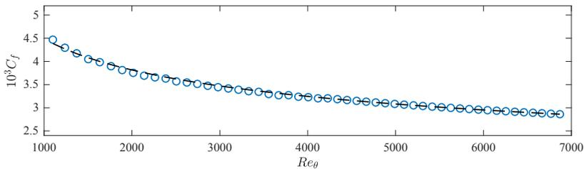
**Fig. 5 Predicted friction coefficients for turbulent boundary layer.** Friction coefficient  $C_f$  as a function of  $Re_\theta$ . Symbols are LLWM and line is the empirical  $C_f$  [49].
