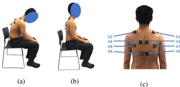
Fig. 1: Experimental setup of static poses. (a) poor posture. (b) natural posture. (c) placement of sEMG sensors.
