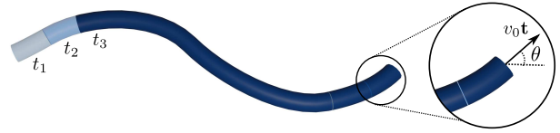
Fig. 1: Schematic illustration of the active directional filament model on a two-dimensional infinite flat plane at three different times: t_1 \leq t_2 \leq t_3 . The active directional filament consists of an active head segment and passive body segments trailing the trajectory of the active head segment. The magnified region defines the velocity, with constant norm v_0 , tangential vector \mathbf{t} and the orientational angle \theta of the active head segment.
