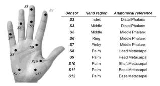
Figure 1: Sensor locations corresponding to mechanoreceptor regions generating thousands of grip forces (expert and novice data), exploited and modeled here.
