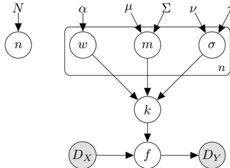
Figure 1: Bayesian Network of our model. The number of mixture components  $n$  is drawn from a uniform prior;  $\alpha$  parameterises a Dirichlet distribution over mixture weights  $w$ ;  $\mu$  and  $\Sigma$  parameterise Gaussians over mixture means;  $\nu$  and  $\tau$  parameterise Log-Normal distributions over mixture scales. Not shown are hyperparameters of the hyper-kernel,  $\lambda$  and  $l$ .
