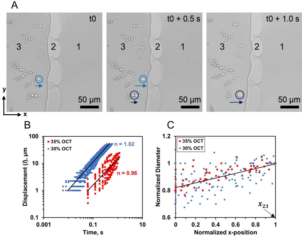
**Figure 12.** Comparison between initial solution compositions. (A) Time-based optical images of water-rich droplet movement in zone 3 with 35 wt-% octanol in solution A. (B) Displacement of water-rich droplets in zone 3 as a function of time with 30 wt-% and 35 wt-% octanol in solution A. (C) Normalized water-rich droplet diameter as a function of normalized x-position in zone 3.
