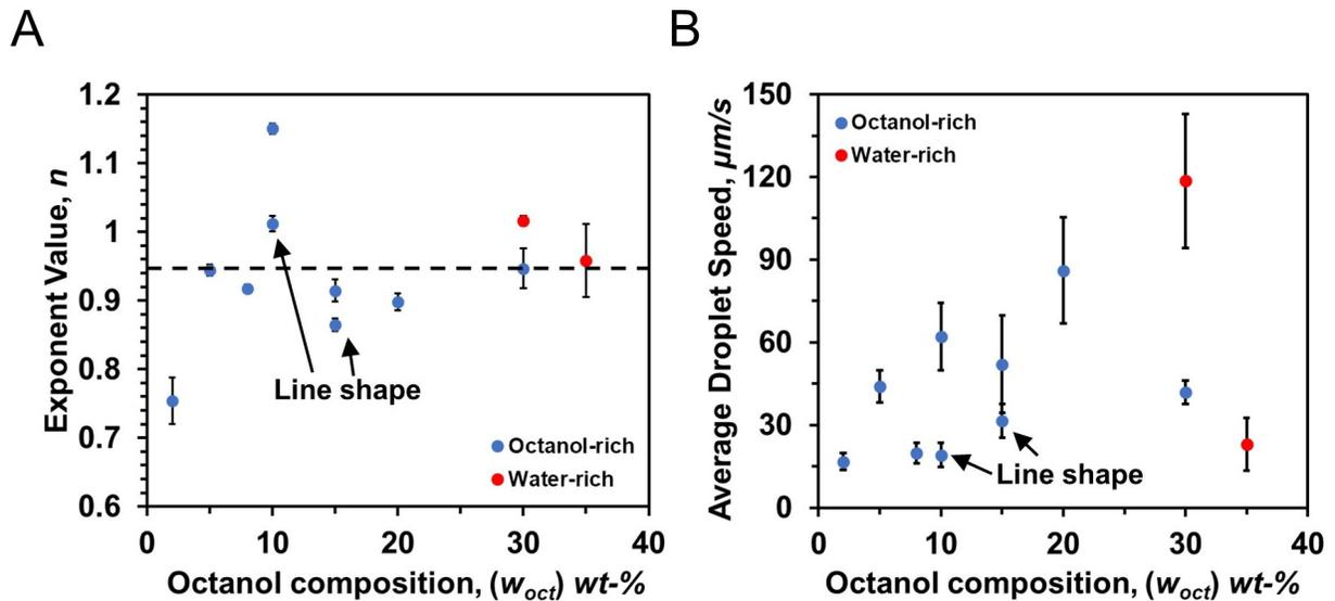
**Figure 14.** (A) Droplet displacement scaling as a function of octanol wt-% in solution A. (B) Average droplet speed as a function of octanol wt-% in solution A. Oil-rich droplets formed from line-shaped protrusions are annotated.
