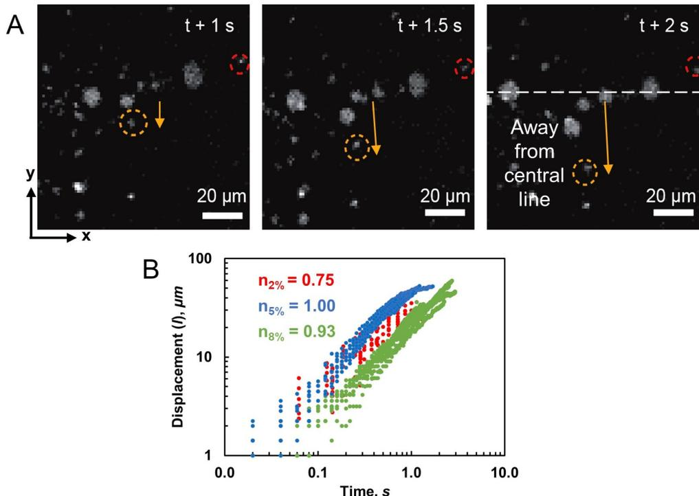
**Figure 4.** (A) Time-based optical images of droplets moving away from a triangular protrusion for solution A with 8 wt-% octanol. The red dotted circle shows a stationary object as a reference. A representative moving droplet is indicated with a yellow dotted circle. (B) Octanol-rich droplet displacement versus time from a stable triangular protrusion for solution A with 2 wt-% (red), 5 wt-% (blue) and 8 wt-% (green) octanol.
