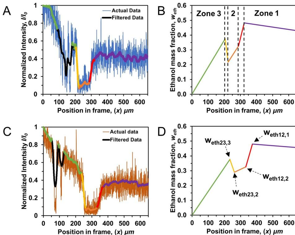
**Figure 8.** Concentration gradients as indicated by fluorescence intensity at  $t_0$  for 30 wt-% octanol in solution A. (A) and (C) Normalized intensity profile as a function of x-position. (B) and (D) Ethanol mass fraction as a function of x-position calculated from intensity profiles. Different colours represent the slope along each zone and boundary.
