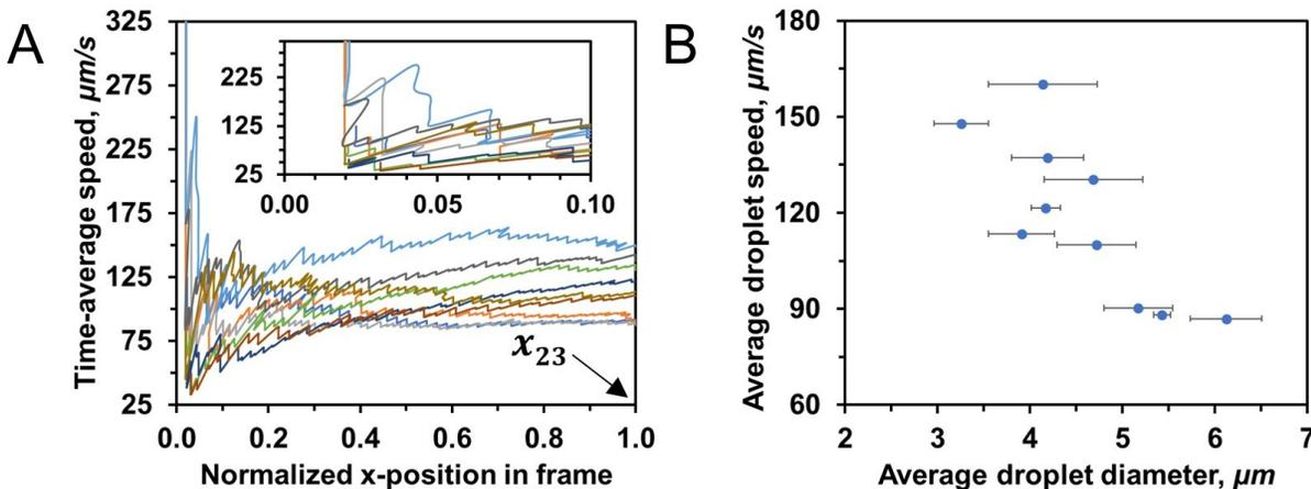
**Figure 11.** (A) Time-averaged droplet speed as a function of normalized droplet displacement. Inset: zoom-in plot of early displacement. (B) Water-rich droplet speed as a function of average droplet size at 30 wt-% octanol composition.
