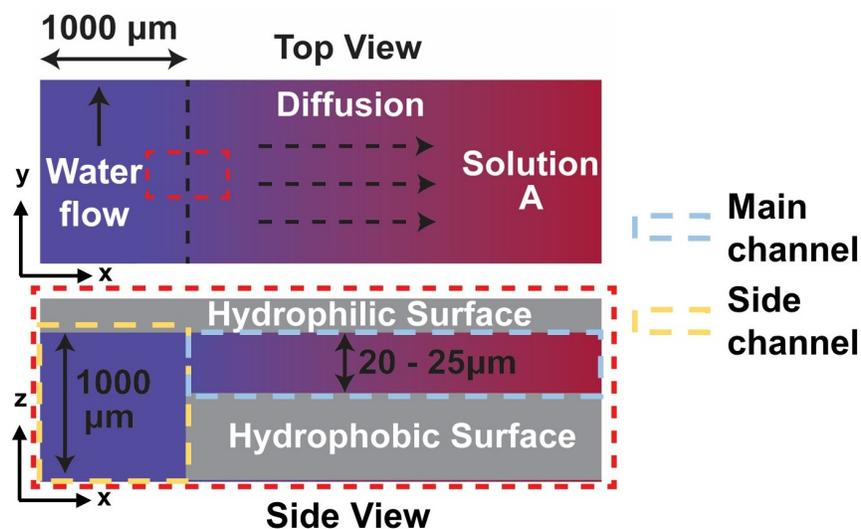
**Figure 2.** Top view and cross-section sketches of the main and side channels of the microchannel. The ternary solution A fills the narrow and wide main channel. The poor solvent water flows in the deep side channel and diffuses transversely into the main channel. Adapted from *Energy Fuels* **2021**, 35, 6, 5194–5205 (<sup>39</sup>). Copyright 2021 American Chemical Society.
