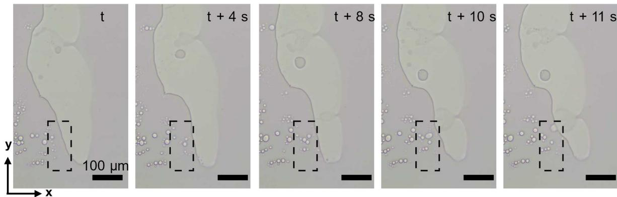
**Figure 13.** Time-based optical images at the 35 wt-% octanol solution composition showing water-rich droplet nucleation, growth and subsequent coalescence.
