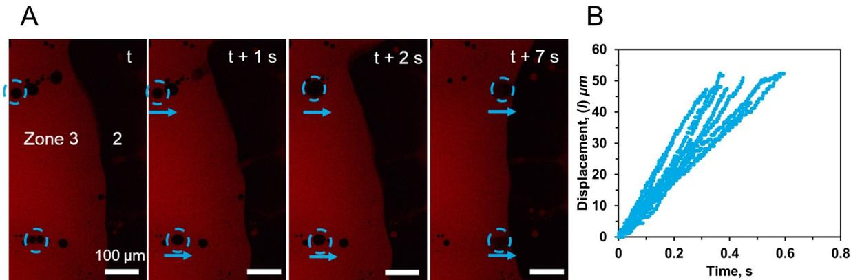
**Figure 10.** (A) Time-based fluorescence image of water-rich droplet movement at the 30 wt-% octanol composition. Dashed circles indicate the movement of two water-rich droplets within zone 3. (B) Displacement of water-rich droplets in zone 3 as a function of time. Each set of dots represents the motion of one droplet measured with a high-speed camera. The final displacement position of each droplet is when they merge with the boundary between zone 2 and 3.
