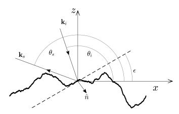
FIG. 1. Rough surface scattering geometry. The nominal incident and scattered wave vector are shown, along with the slope angle,  $\epsilon$ , at the origin, and the unit normal vector at that point, which is defined to point out of the acoustic domain, which is defined as the upper medium.
