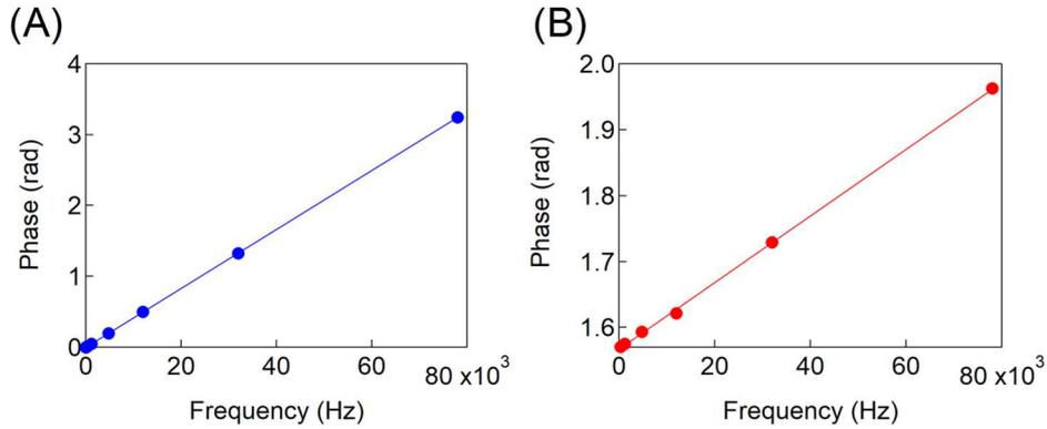
**Fig. S3** Phase delays observed in the response of (A) AOD and (B) PID feedback controller to the sinusoidal input signal. (A, B) Phase delays were proportional to the frequency as  $\omega\tau_{\text{AOD}}$  and  $\omega\tau_{\text{contr}}$ , respectively. From the linear fit to the data (solid lines), we obtained  $\tau_{\text{AOD}} = 6.6 \times 10^{-6}$  s and  $\tau_{\text{contr}} = 8.1 \times 10^{-7}$  s.
