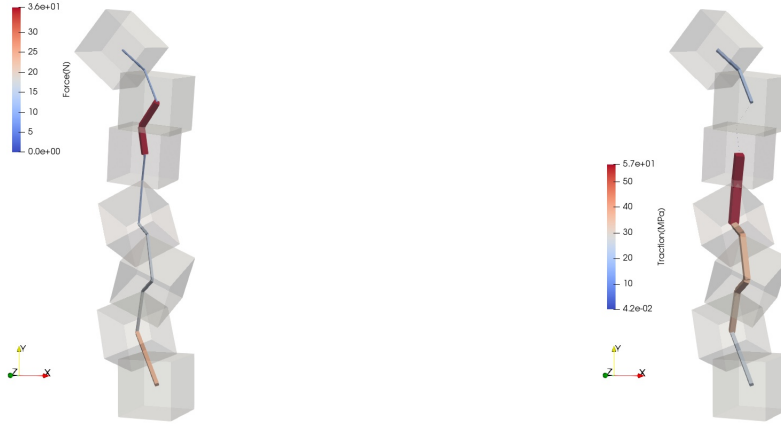
Figure 16: Topple stack: Force chain network (left) and traction chain network (right) for a septenary particle system.
