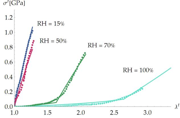
FIG. A8. Theoretical (continuous lines) *vs* experimental (dots) stress-stretch curves for *Argiope trifasciata* spider fibers at different humidity and  $T = 55^\circ\text{C}$  (reproduced from [29]). Here  $k^h = 0.99$  GPa,  $k^s = 18.2$  MPa,  $\mu = 0.01$  MPa,  $c_1 = 1.18$ ,  $c_2 = 1.1$ ,  $\alpha = 0.0085$ ,  $m_f/m_o = 0.162$ ,  $s = 5.5$ ,  $\lambda_c^s = 1.57$ ,  $\lambda_{lim} = 1.27$ ,  $\text{RH}_c = 66.5\%$ .
