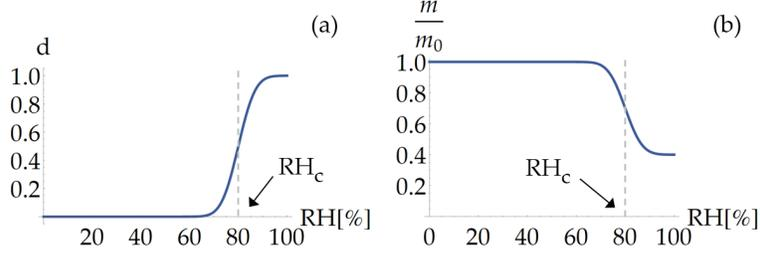
FIG. A1. (a) Damage parameter  $d$  representing the percentage of broken links as a function of humidity. (b) Influence of the relative humidity on the number of H-bonds with respect to the initial number of H-bond. Here  $\text{RH}_c = 80\%$ ,  $s = 5.5$  and  $m_f/m_o = 0.4$ .
