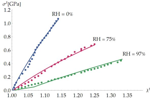
FIG. A7. Theoretical (continuous lines) *vs* experimental (dots) stress-stretch curves for *Nephila clavata* fibers at different humidity and  $T = 25$  °C (reproduced from the experiments at strain rate of  $3.3 \times 10^{-3} s^{-1}$  in [31]). Here  $k^h = 5.6$  GPa,  $k^s = 1.47$  GPa,  $\mu = 1.1$  MPa,  $c_1 = 1.35$ ,  $c_2 = 1.46$ ,  $\alpha = 0.009$ ,  $m_f/m_o = 0.878$ ,  $s = 3$ ,  $\lambda_c^s = 4.6$ ,  $\lambda_{lim} = 1.25$ ,  $RH_c = 80\%$ .
