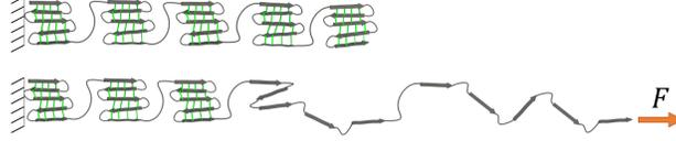
FIG. A3. Cartoon of a chain of the hard region undergoing a folded  $\rightarrow$  unfolded transition when subjected to a force.
