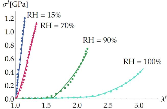
FIG. 3. Theoretical (continuous lines) *vs* experimental (dots, reproduced from [18]) stress-stretch curves for *Argiope trifasciata* spider fibers at different RH and  $T = 20$  °C. Here  $k^h = 2.2$  GPa,  $k^s = 13.5$  MPa,  $\mu = 0.14$  MPa,  $c_1 = 1.3$ ,  $c_2 = 0.87$ ,  $\alpha = 0.0094$ ,  $s = 8.5$ ,  $m_f/m_o = 0.12$ ,  $\lambda_c^s = 1.62$ ,  $\lambda_{lim} = 1.34$ .
