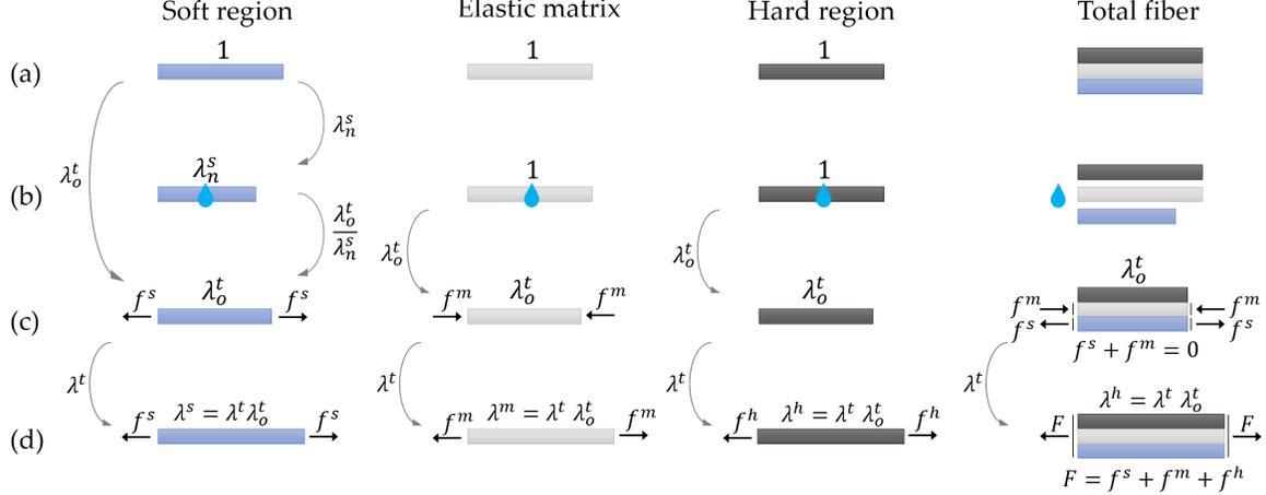
FIG. A5. Scheme of the evolution of the configurations of the different composing phases and of the whole fiber: (a) dry natural configuration, (b) humid condition without external forces where selfstresses (reported in (c)) are induced by kinematic compatibility, (d) non zero external force configurations.
