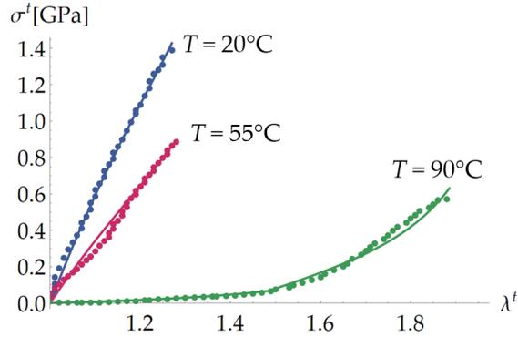
FIG. 5. Theoretical (continuous lines) *vs* experimental (dots) stress-stretch curves for *Argiope trifasciata* spider fibers at different temperature at fixed RH = 50% (reproduced from [29]). Here  $T_g = 84$  °C,  $k^h = 3.83$  GPa,  $k^s = 32.7$  MPa,  $\mu = 2$  MPa,  $c_1 = 1.36$ ,  $c_2 = 1.25$ ,  $\alpha = 0.00995$ ,  $s = 4.5$ ,  $m_f/m_o = 0.345$ ,  $\lambda_c^s = 1.49$ ,  $\lambda_{lim} = 1.27$ .
