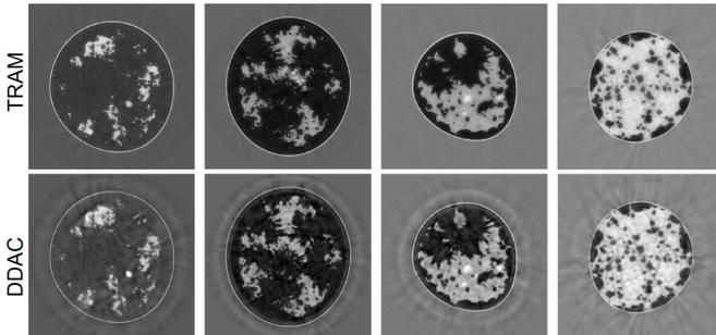
Fig. 10. Case study 1: Reconstructed SOS images corresponding to the same phantoms shown in Fig. 9 using TRAM (top row) and DDAC (bottom row). From left to right: breast type A-D. The unit is  $(mm/\mu s)$ .
