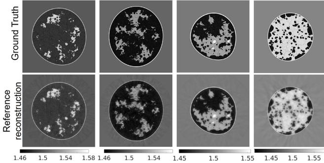
Fig. 9. Reference images: Ground truth (top row) and reconstructed (bottom row) SOS maps. From left to right: breast type A-D. The unit is  $(mm/\mu s)$ .
