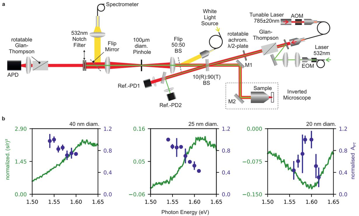
FIG. 1. Experimental setup with photothermal signal optimization: Panel **a** shows the optical setup. Panel **b** shows sections of white-light scattering spectra normalized to the reflection on the glass slide ( $(s/r)^2$ , green line) and the corresponding relative photothermal amplitude  $A_{PT}$  values (blue dots) obtained while varying the tunable laser's wavelength for NRs with various diameters.
