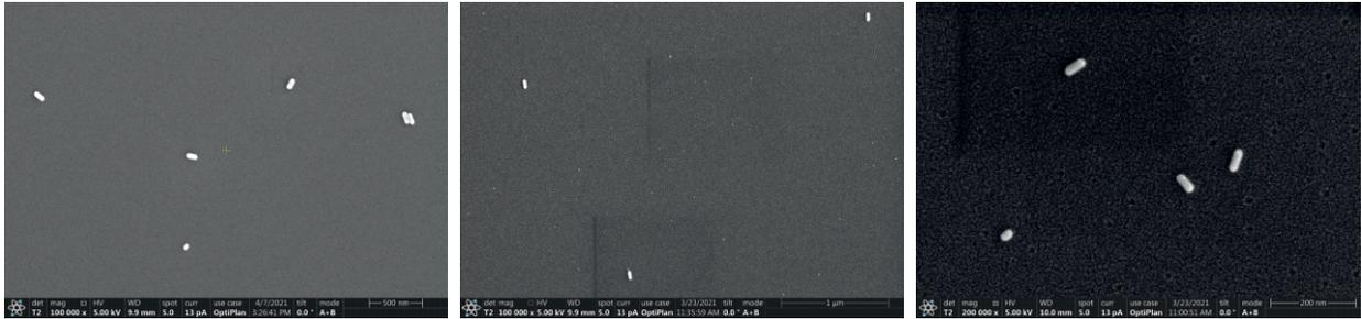
Figure S 2. Example SEM micrographs showing nanorod samples with average diameters of 40, 25, and 20 nm (left to right). NRs have various aspect ratios and suited candidates are selected based on white-light scattering spectra.
