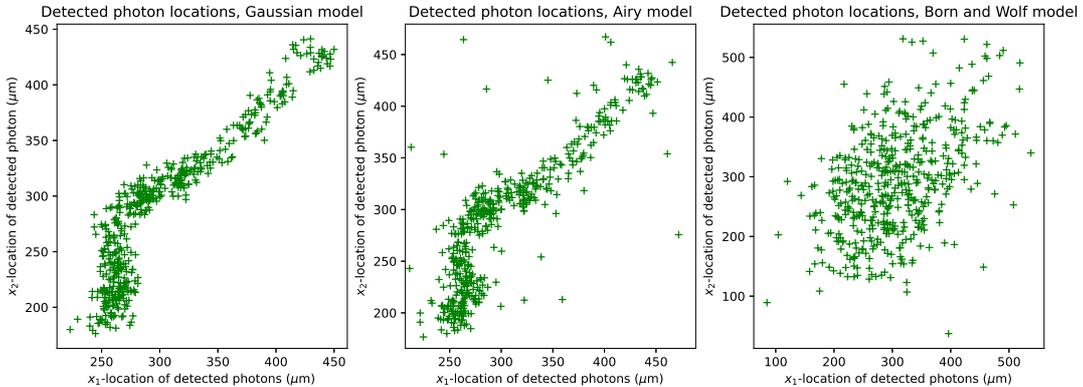
**Figure 3:** Detected photon locations of a moving molecule with stochastic trajectory for the 2D Gaussian (left), Airy (middle) profiles and Born and Wolf model (right).
