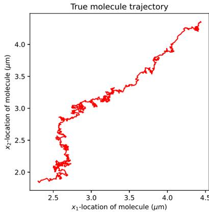
**Figure 2:** Trajectory of a molecule in the object space with stochastic trajectory described in (2.6) and with diffusion and drift coefficients  $\sigma^2 = 1 \text{ } \mu\text{m}^2/\text{s}$  and  $b = -10 \text{ s}^{-1}$ , respectively. The molecule moves during an interval of  $[0, 0.1]$  seconds and its initial location is Gaussian distributed with mean  $x_0 = (4.4, 4.4)^\top \text{ } \mu\text{m}$  and covariance  $P_0 = 10^{-2} \mathbb{I}_{2 \times 2} \text{ } \mu\text{m}^2$ .
