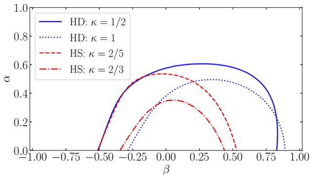
FIG. 6. Plane  $\alpha$  vs  $\beta$  showing the locus  $k_{\perp} = k_{\parallel}$  for HD ( $\kappa = \frac{1}{2}$  and 1) and HS ( $\kappa = \frac{2}{5}$  and  $\frac{2}{3}$ ). In each case, the longitudinal heat mode is the most unstable one ( $k_{\parallel} > k_{\perp}$ ) in the region below the locus.
